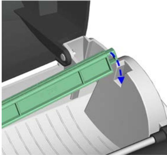
(B) Installing the label supply hub
