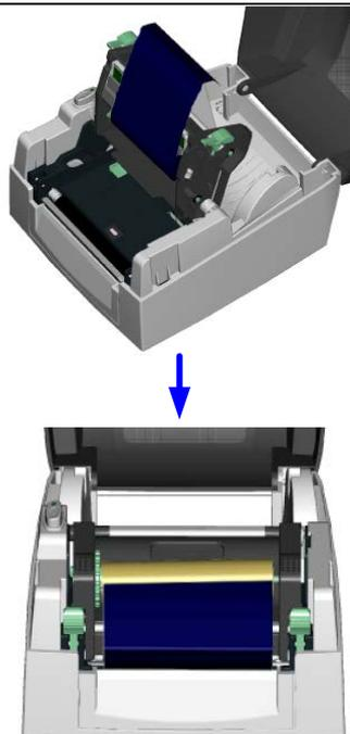
7. Turn the ribbon feed mechanism to tighten the ribbon until it has no wrinkles.
